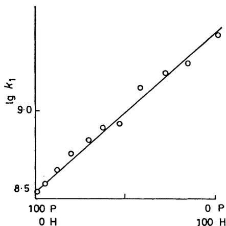
FIGURE 3  $\lg k$ , as a function of the composition of hexane(H)-propanol(P) mixture
