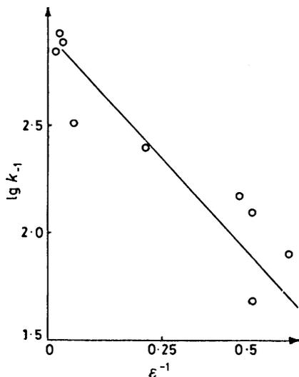
FIGURE 1  $k_{-1}$ , as a function of the dielectric constant of the solvent
