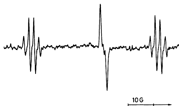
FIGURE 3 E.s.r. spectra of \text{CH}_3\text{N}=\dot{\text{C}}\text{OSiMe}_3 and \text{CF}_3\dot{\text{C}}(\text{OMe})\text{OSiMe}_3 generated by photolysis at 163 K of a cyclopropane solution containing \text{MeNCO} (2.1M), \text{CF}_3\text{C}(\text{O})\text{OMe} (1.3M), \text{Me}_3\text{SiH} , and \text{Bu}^t\text{OOBu}^t . The lines of \text{CF}_3\dot{\text{C}}(\text{OMe})\text{OSiMe}_3 corresponding to M_1(3\text{F}) \pm 1/2 are broadened beyond the limit of detectability (see text).
