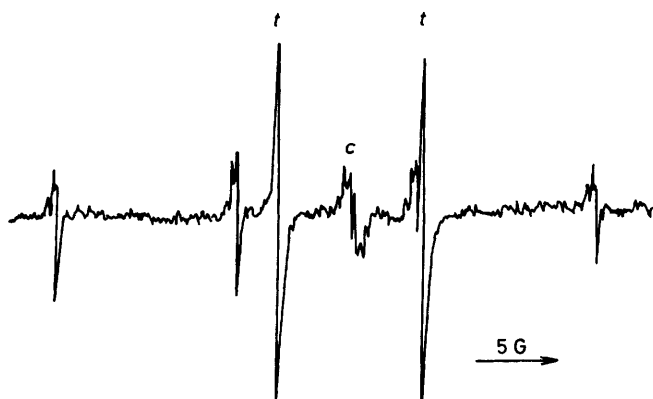
Figure 2. E.s.r. spectrum observed from the photolysis of cyclopropyl t-butyl ketone in \text{CF}_2\text{Cl}_2 at 143 K, showing the doublet of the trans -cyclopropylacyl radical ( t ) and the multiplet of the cis -cyclopropylacyl radical ( c ) superimposed in the signals of the t-butyl radical
