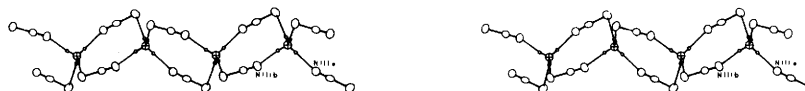
Figure 6. Stereoview of the cation-anion chains in the (NH_4SCN)_2(I) crystals. Atoms are represented by 30% thermal ellipsoids. The crystallographic c axis is horizontal, and the b axis vertical in the plane of the paper
