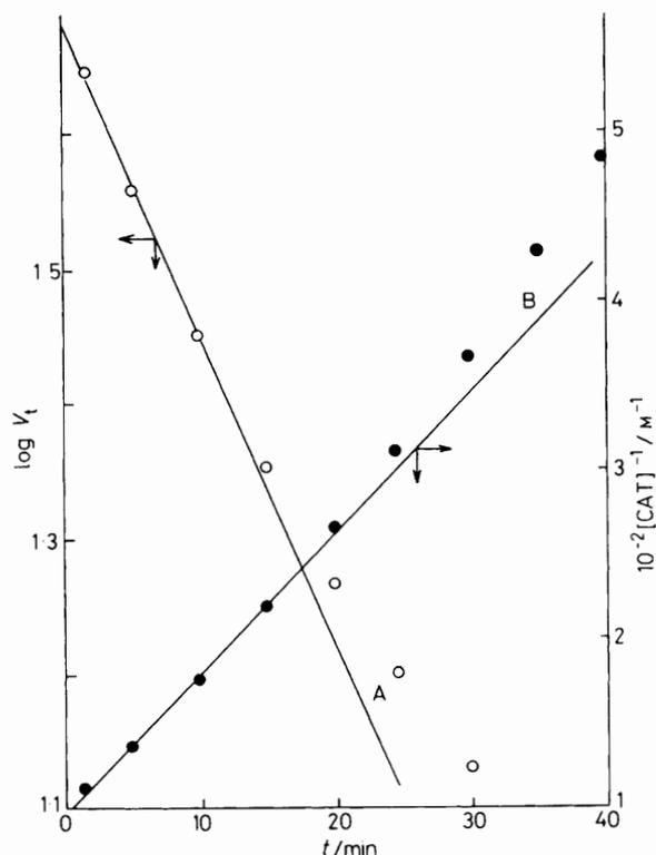
Figure 1. A, Plot of  $\log V_t$  versus time; B plot of  $[CAT]^{-1}$  versus time. [CAT]  $9.4 \times 10^{-3}$ ; [AA] 0.05;  $[H^+]$  0.10;  $[RNH_2]$  0.01;  $\mu$  0.14M; temp.  $30^\circ C$
