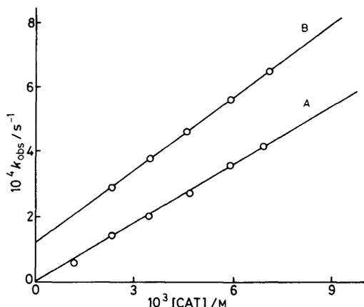
**Figure 2.** Plot of  $k_{\text{obs}}$  versus  $[\text{CAT}]$  at 30 °C and  $\mu$  0.14M: A,  $[\text{AA}]$  0.04;  $[\text{H}^+]$  0.10;  $[\text{RNH}_2]$  0.01M; B,  $[\text{AA}]$  0.04;  $[\text{H}^+]$  0.10;  $[\text{RNH}_2]$  0.01;  $[\text{Cl}^-]$  0.015M
