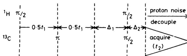
Figure 1. Pulse sequence for 2D C–H correlation spectroscopy
