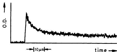
Figure 1. Trace of optical absorption at 500 nm versus time from pulse-irradiated, N 2 O-saturated, pH ca. 4 solution containing 5 × 10 -3 M-KSCN and 2 × 10 -3 M-CH 3 SSCH 3 .
