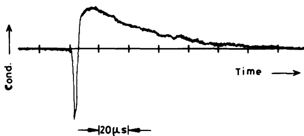
Figure 5. Conductivity vs. time traces in pulse-irradiated deoxygenated ( N_2 -sat.) solutions of [4.4.4]^{2+} ( 5 \times 10^{-4} \text{ mol dm}^{-3} ) at pH 3.9; the initial negative spike is of an electronic nature
