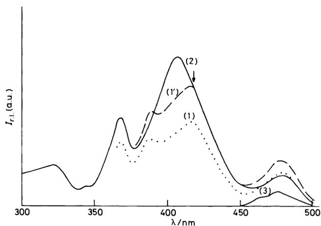
**Figure 4.** Corrected r.l. excitation spectra of preirradiated DCA-DMN in acetonitrile at 77 K;  $\lambda_{em} = 530$  nm (peak of the emission in Figure 3): (1) deaerated sample; (2) sample saturated with  $O_2$ ; (1') curve (1) normalized at point of curve (2) marked by arrow; (3) difference between curve (1') and curve (2);  $DCA^{2-}$
