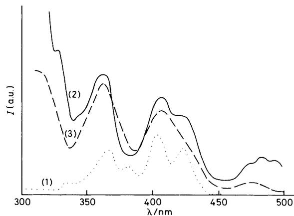
**Figure 6.** Corrected excitation spectra of DCA-DMN in various solvents: (1)  $\lambda_{\text{em}}$  430 or 460 nm ( $^1\text{DCA}^*$  emission) at 300 K (similar to the DCA optical absorption spectrum); (2)  $\lambda_{\text{em}}$  *ca.* 540 nm [ $^1(\text{DCA} \cdots \text{DMN})^*$  emission] at 300 K in acetonitrile; (3)  $\lambda_{\text{em}}$  430, 460, or 520 nm at 77 K
