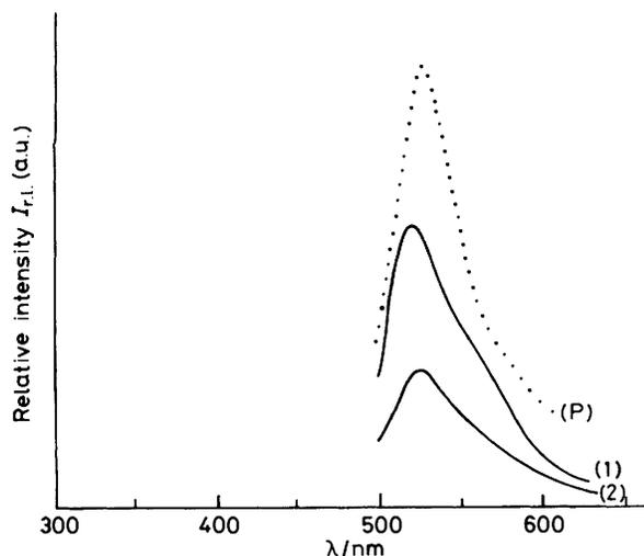
**Figure 1.** The r.l. emission spectrum  $I_{r,i} = f(\lambda_{em})\lambda_b$  of preirradiated DCA-DMN in acetonitrile at 77 K;  $\lambda_b$  480 nm: (1) 5 min after the irradiation is cut off; (2) after bleaching with  $\lambda_b = 480$  nm for 30 min; (P) phosphorescence of DCA-DMN solutions
