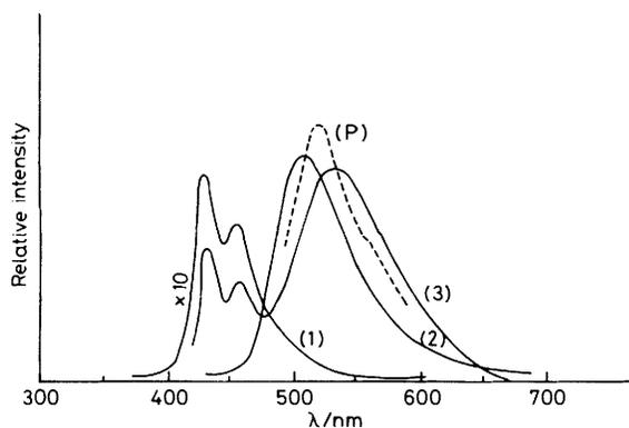
**Figure 5.** Emission spectra of deaerated solutions of DCA-DMN in acetonitrile at (1) 300 K and (2) 77 K and (3) in benzene at 300 K ( $\lambda_{\text{ex}} = 420$  nm); (P) phosphorescence (see text);  $[\text{DCA}] = 10^{-5}\text{M}$ ,  $[\text{DMN}] = 6.4 \times 10^{-2}\text{M}$
