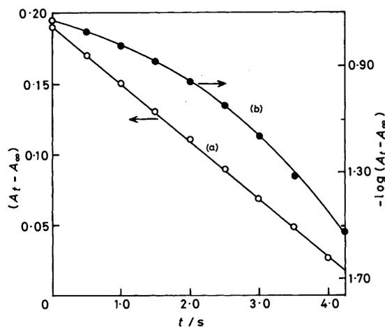
**Figure 1.** Representative kinetic plots of (a)  $(A_t - A_\infty)$  versus time and (b)  $-\log(A_t - A_\infty)$  against time for the oxidation of fructose by  $\text{Co}^{\text{III}}\text{M}$  at  $60^\circ\text{C}$ .  $[\text{Co}^{\text{III}}\text{M}] = 2 \times 10^{-4} \text{ mol dm}^{-3}$ ,  $[\text{Fru}] = 0.80 \text{ mol dm}^{-3}$ ,  $[\text{NaClO}_4] = 1.0 \text{ mol dm}^{-3}$ ,  $[\text{H}^+] = 0.10 \pm 0.01 \text{ mol dm}^{-3}$
