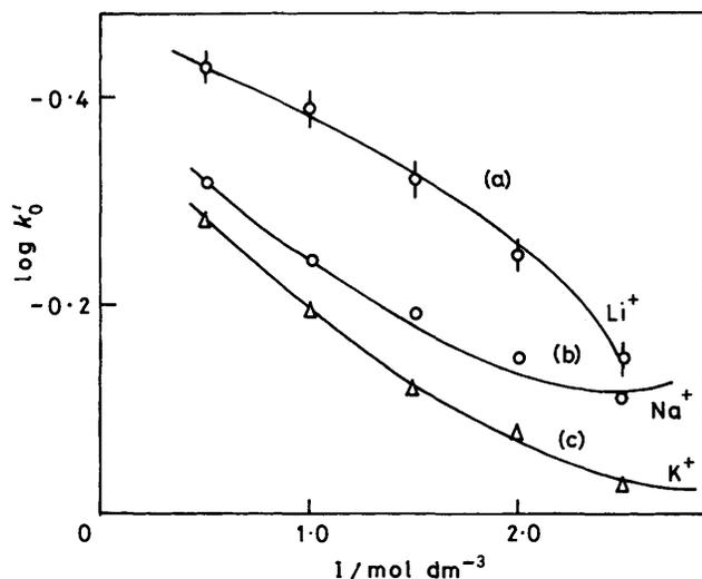
**Figure 3.** Brønsted-Christiansen-Scatchard plots showing the dependence of  $\log k'_0$  on ionic strength for the electron-transfer reaction between  $\text{Co}^{\text{III}}\text{M}$  and mannose at  $60^\circ\text{C}$  in (a)  $\text{LiNO}_3$ , (b)  $\text{NaClO}_4$ , and (c)  $\text{KNO}_3$  media
