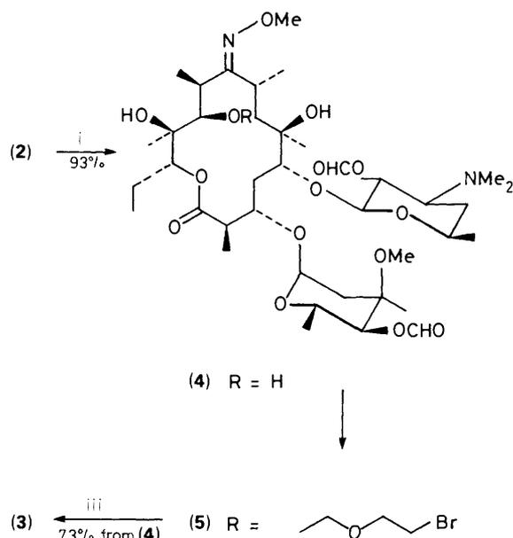
**Scheme.** Reagents: i, AcOCHO, 4-dimethylaminopyridine,  $\text{CH}_2\text{Cl}_2$ ; ii,  $\text{BrCH}_2\text{CH}_2\text{OCH}_2\text{Cl}$ , 2,6-lutidine, *N,N*-dimethylformamide; iii,  $\text{HNMe}_2$ , *N,N*-dimethylformamide,  $60^\circ\text{C}$ . The yields of each step are given.
