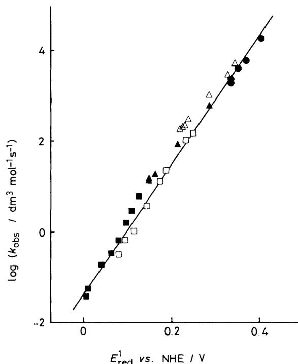
**Figure 4.** Plots of  $\log k_{\text{obs}}$  vs. the one-electron reduction potentials of Q ( $E_{\text{red}}^1$ ) for the reduction of *p*-benzoquinone derivatives by  $\text{AcrH}_2$  in  $\text{H}_2\text{O}$ -EtOH (5:1 v/v) at 298 K. The symbols are the same as those used in Figure 2.
