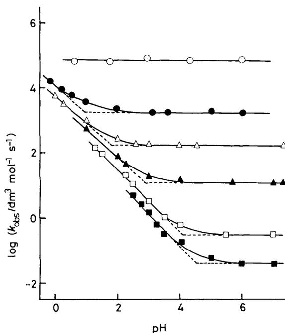
**Figure 2.** Plots of  $\log k_{obs}$  vs. pH for the reduction of TCNQ (○), *p*-chloranil (●), 2,6-dichloro-*p*-benzoquinone (△), chloro-*p*-benzoquinone (▲), *p*-benzoquinone (□), and methyl-*p*-benzoquinone (■) in H<sub>2</sub>O–EtOH (5:1 v/v) at 298 K.
