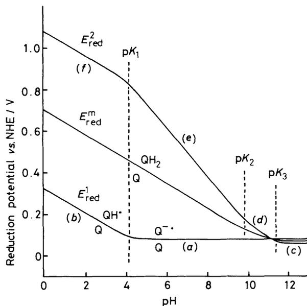
**Figure 1.** Dependence of the reduction potentials of *p*-benzoquinone (Q) in H<sub>2</sub>O.<sup>11</sup> The lower line is the one-electron reduction process of Q. The upper line is the one-electron reduction process of Q<sup>-•</sup> and QH<sup>•</sup>. The middle line is the two-electron reduction process of Q [equation (1)].
