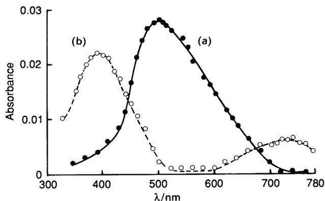
**Figure 3.** Transient optical absorption spectrum on pulse radiolysis of  $O_2$ -saturated aq. (pH 1.5) TDPA ( $2.8 \times 10^{-2} \text{ mol dm}^{-3}$ ) and  $I^-$  ( $9.0 \times 10^{-5} \text{ mol dm}^{-3}$ ) (a) immediately; (b)  $7 \mu\text{s}$  after the pulse.
