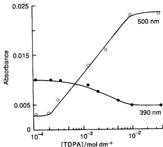
**Figure 2.** Variation in the absorbance of transient bands formed on pulse radiolysis of  $O_2$ -saturated aq. solutions (pH 1.5) at different concentrations of TDPA.
