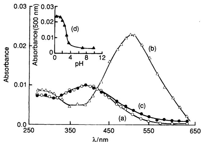
**Figure 1.** Transient optical absorption spectrum obtained on pulse radiolysis of  $O_2$ -saturated aq. (a) TDPA ( $2.8 \times 10^{-3} \text{ mol dm}^{-3}$ , pH 6.0); (b) TDPA ( $2.8 \times 10^{-2} \text{ mol dm}^{-3}$ , pH 1.5); (c) TDPA ( $2.8 \times 10^{-4} \text{ mol dm}^{-3}$ , pH 1.5); (d) variation of absorbance of 500 nm band of  $(\text{TDPA})_2^+$  formed on pulse radiolysis of  $O_2$ -saturated aq. TDPA ( $2.8 \times 10^{-2} \text{ mol dm}^{-3}$ ) with pH.
