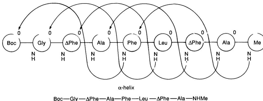
Fig. 7. The conformation compatible with NMR data for heptapeptide **8** in  $\text{CDCl}_3$ .
