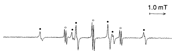
Fig. 1 EPR spectra of \cdot\text{CH}_2\text{OH} (◦) and \text{HOCH}_2\text{CH}_2\dot{\text{C}}\text{HCO}_2\text{H} (•) produced from the addition of \cdot\text{CH}_2\text{OH} to acrylic acid at pH 2 ( [\text{Ti}^{\text{III}}] 1.67 \times 10^{-3} , [\text{H}_2\text{O}_2]_0 1.67 \times 10^{-2} , [\text{MeOH}]_0 1.7 , [\text{acrylic acid}]_0 3 \times 10^{-3} \text{ mol dm}^{-3} ).
