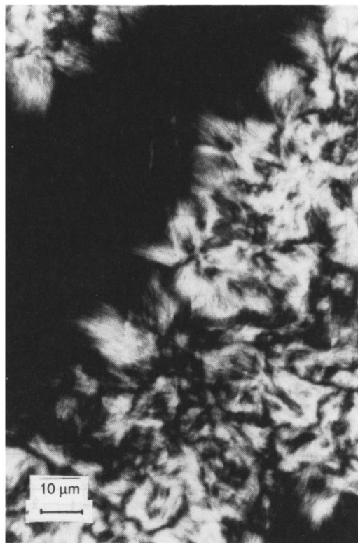
Fig. 7 Optical micrograph of 2'2C_{18} ( 150.7\ mg\ g^{-1} ) in carbon disulfide under crossed Nicol prisms at room temperature. Under these conditions the sample is in the gel phase.
