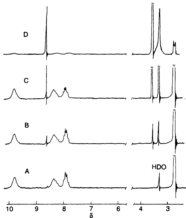
Fig. 5 Spectra which result after heating 13A and 13B in boiling (\text{CD}_3)_2\text{SO} . A, The mixture of the proposed intermediates before heating. B, After heating for 5 min. C, After heating for 10 min. D, After heating for 20 min. Only 8 is visible after 30 min.
