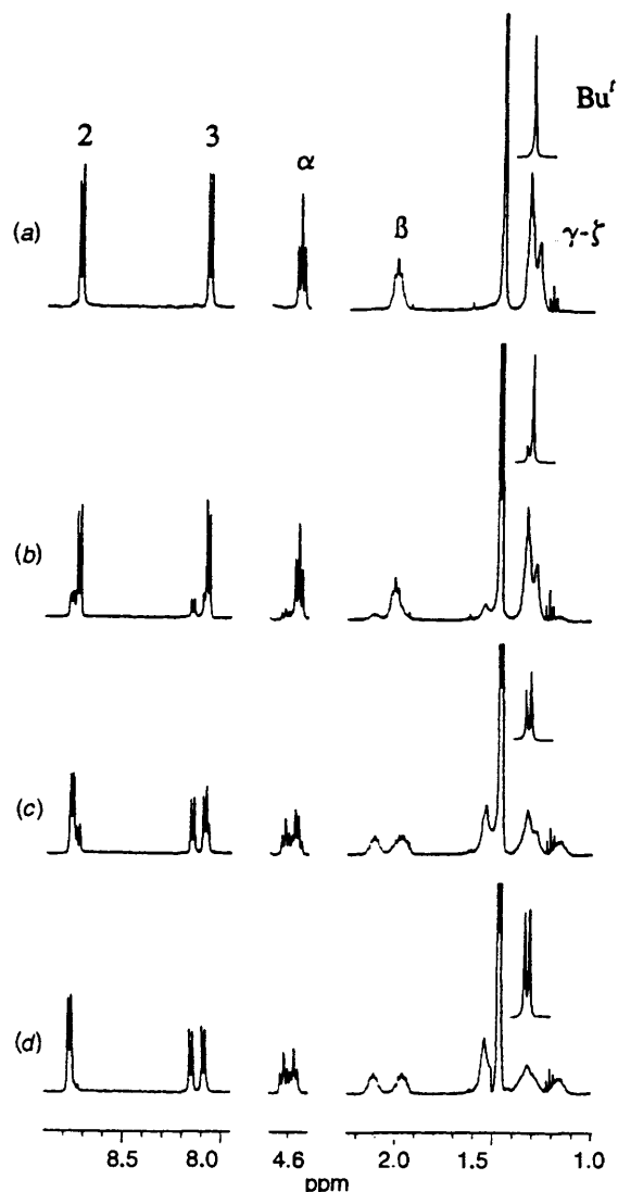
Fig. 1 ^1\text{H} NMR spectra (400 MHz) of the formation of the [2]pseudorotaxane \{\text{tbp}(\text{CH}_2)_{10}\text{tbp}\cdot\alpha\text{-CD}\}^{2+} , recorded (a) 2 min, (b) 20 min, (c) 150 min and (d) 6 h after mixing [\text{tbp}(\text{CH}_2)_{10}\text{tbp}]^{2+} ( 5.0 \times 10^{-3} mol \text{dm}^{-3} after mixing) with \alpha -cyclodextrin ( 5.0 \times 10^{-2} mol \text{dm}^{-3} after mixing) in \text{D}_2\text{O} (0.10 mol \text{dm}^{-3} NaCl) at 25 °C
