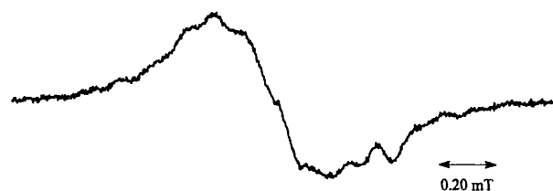
Fig. 4 EPR spectrum, obtained by UV irradiation of a solution of dibenzofuran ( 10 \text{ mmol dm}^{-3} ) and thallium(III) trifluoroacetate ( \approx 20 \text{ mmol dm}^{-3} ) in HFP at 22^\circ\text{C}
