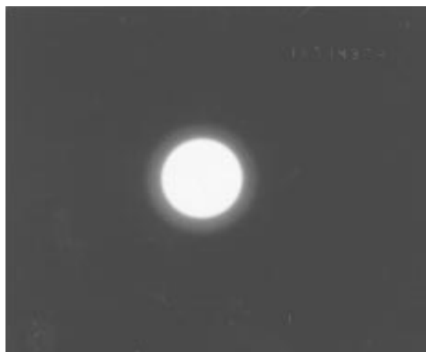
Fig. 6 Electron diffraction photograph of C_{60} sol; 0.11 \text{ mg ml}^{-1} C_{60} sol was spread on a collodion film substrate with graphite powder
