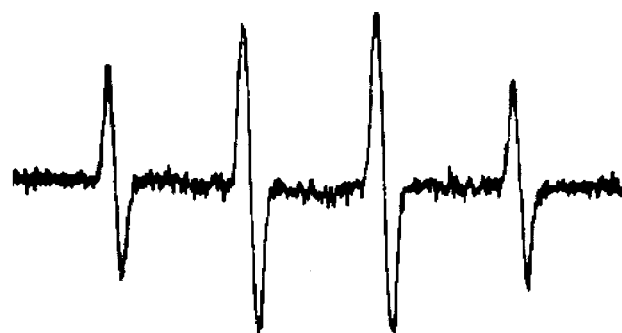
Fig. 3 EPR of DMPO-OR spin adduct (R from AAPH)
