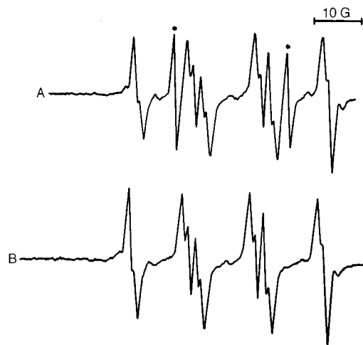
Fig. 3 (A) A composite EPR spectrum consisting of ^{14}\text{N} -DMPO-OOH and ^{15}\text{N} -D 17 -4-MAL-TEMPO (designated with a *). Superoxide was generated using a hypoxanthine/xanthine oxidase in sodium phosphate buffer (0.1 M, pH 7.8), as a source of this free radical. (B) The same conditions as in (A) except ^{15}\text{N} -D 17 -4-MAL-TEMPO was not present in the reaction mixture. Microwave power was 20 mW, modulation frequency was 100 kHz with an amplitude of 1.0 G, sweep time was 12.5 G min -1 , and the receiver gain of 5 \times 10^3 with a response time 1.0 s.
