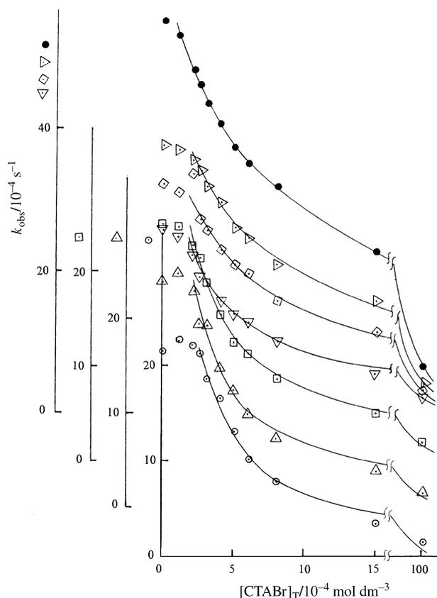
Fig. 1 Effects of [CTABr]<sub>T</sub> on pseudo-first-order rate constants ( $k_{obs}$ ) for alkaline hydrolysis of PTH at 35 °C and [NaOH] = 0.005 (O), 0.02 (Δ), 0.05 (□), 0.1 (▽), 0.3 (◇), 0.5 (▷) and 0.8 mol dm<sup>-3</sup> (●). The solid lines are drawn through the calculated data points using eqn. (3) and unknown parameters,  $k_M$  and  $K_S$ , listed in Table 1.
