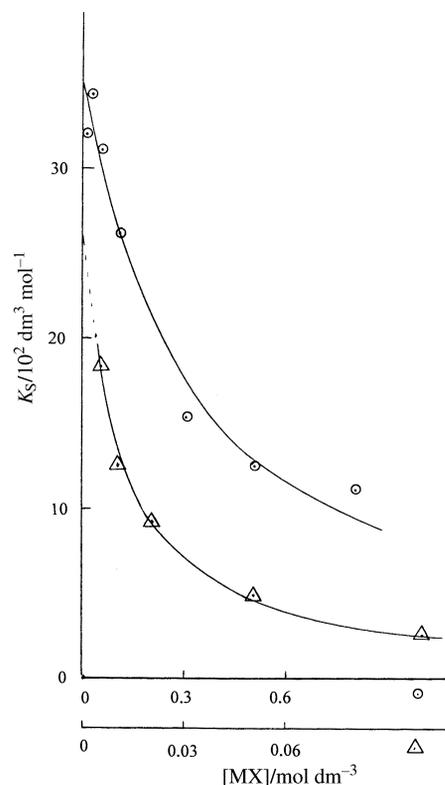
**Fig. 2** Plots showing the dependence of CTABr micellar binding constants ( $K_S$ ) of ionized PTH upon  $[\text{MX}]$  where  $\text{MX} = \text{NaOH}$  (O) and  $\text{NaBr}$  ( $\Delta$ ). The solid lines are drawn through the calculated data points using eqn. (7) and unknown parameters,  $K_S^0$  and  $\Psi$ , mentioned in the text.
