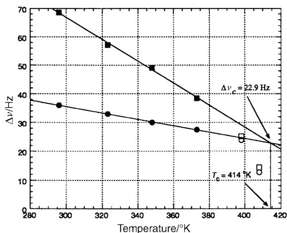
Fig. 4 Temperature dependence for the two pairs of protons that coalesce at 6.91 (●, correlation coefficient,  $R = 0.999$ ) and 6.74 (■,  $R = 0.998$ ) ppm. Only those data have been included in the regression analysis where the individual peaks do not significantly overlap.
