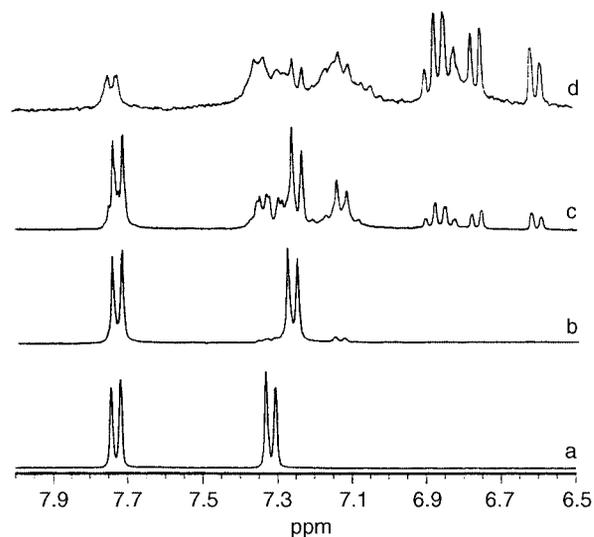
**Fig. 1** Aromatic region of  $^1\text{H}$  NMR spectrum of *L-p*-boronophenylalanine in  $\text{DMSO-}d_6$  with (a) 10%  $\text{D}_2\text{O}$ , (b) 5%  $\text{D}_2\text{O}$ , (c) 1%  $\text{D}_2\text{O}$  and (d)  $\text{DMSO-}d_6$  only.
