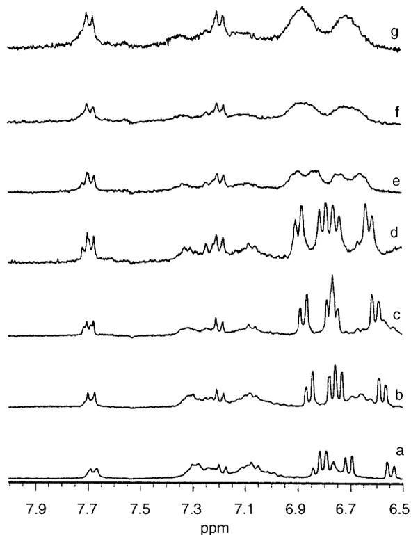
Fig. 3 Aromatic region of VT  $^1\text{H}$  NMR spectrum of *L-p*-BPA in  $\text{DMSO-}d_6$  (18 mM) at (a) 22 °C, (b) 50 °C, (c) 75 °C, (d) 100 °C, (e) 125 °C, (f) 135 °C and (g) 140 °C.
