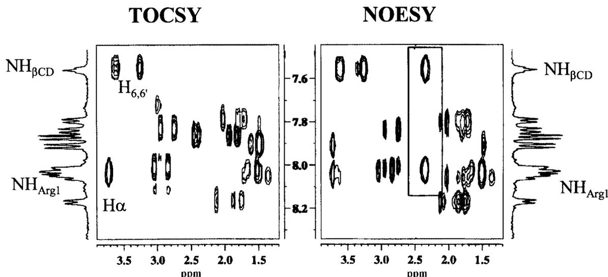
Fig. 4 Partial contour plots (310 K; 500.13 MHz; *d*<sub>6</sub>-DMSO) of TOCSY and NOESY experiments (80 and 200 ms mixing time at 10 and 18 dB attenuation, respectively) performed on samples containing 2.5 mmol dm<sup>-3</sup> of **6a**. Area of inter-residue C<sub>*α*</sub>H<sub>*i*</sub>/NH<sub>*i*+1</sub> cross-peaks.
