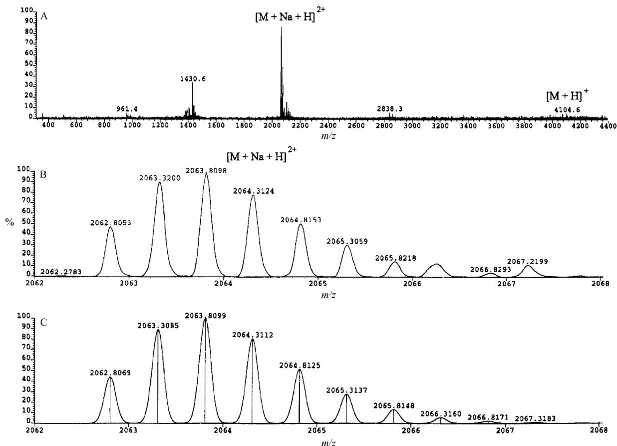
**Fig. 2** ESI-MS spectrum obtained for **8b** (A) and isotope profile measured by ESI-HRMS at  $m/z = 2063$  (B) and calculated (C) for  $C_{167}H_{265}N_{20}NaO_{95}S[M + Na + H]^{2+}$ .
