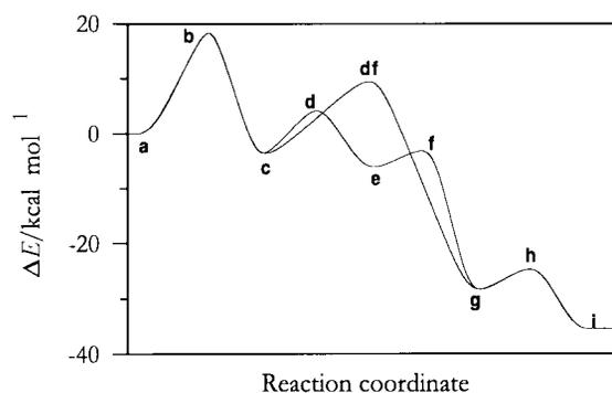
**Fig. 3** Energy profile of the acylation process.
