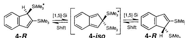
Scheme 2 Scrambling of the trimethylsilyl groups in 4 , as a result of [1,5]-silicon shifts. One silicon group is arbitrarily marked with an asterisk (*) to aid in monitoring its position throughout the migratory process.
