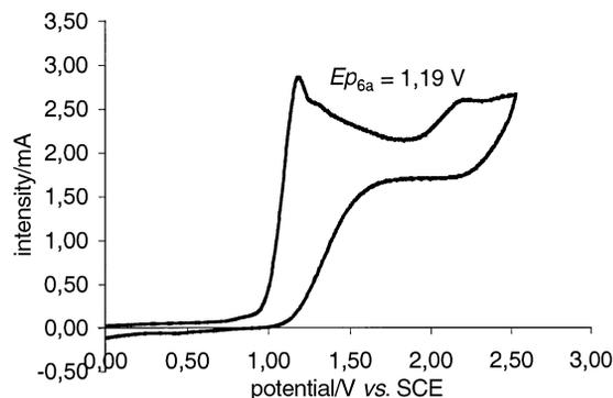
**Fig. 3** Voltammetric investigations of compound **6a** in  $\text{CH}_3\text{CN} + \text{NEt}_4\text{BF}_4$  (0.5 M), scan rate =  $50 \text{ mV s}^{-1}$ .
