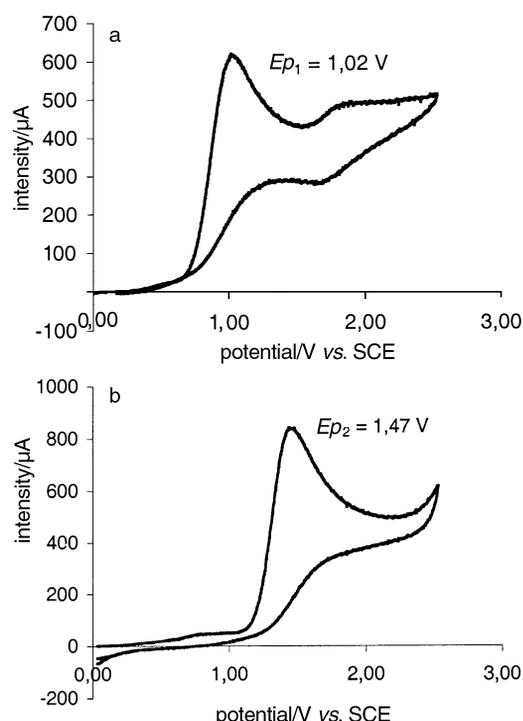
Fig. 1 Voltammetric investigations of compounds **1** (a) and **2** (b) in  $CH_3CN + NEt_4BF_4$  (0.5 M), scan rate =  $50$   $mV s^{-1}$ .
