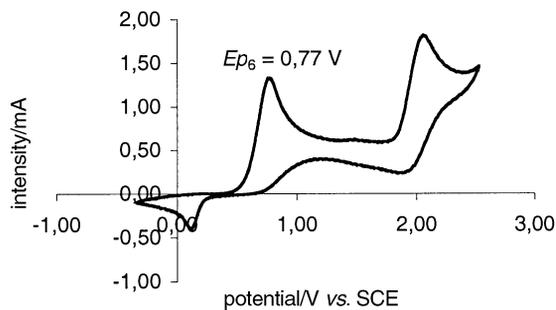
**Fig. 2** Voltammetric investigations of compound **6** in  $\text{CH}_3\text{CN} + \text{NEt}_4\text{BF}_4$  (0.5 M), scan rate =  $50 \text{ mV s}^{-1}$ .
