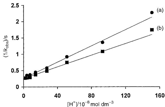
**Fig. 4** Reciprocal plot of  $1/k_{\text{obs}}$  against  $[\text{H}^+]$  for the reactions of (a) *S*-nitrosopenicillamine and (b) *S*-nitrosocysteine with sulfite.
