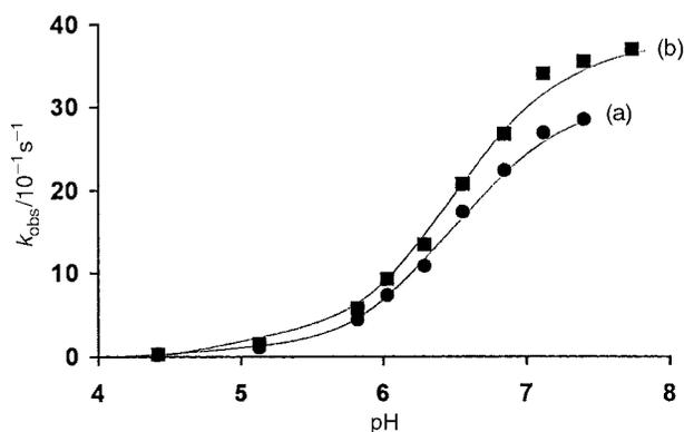
**Fig. 3** Values of  $k_{\text{obs}}$  as a function of pH for the reaction of (a) *S*-nitrosopenicillamine and (b) *S*-nitrosocysteine (both  $2.5 \times 10^{-4} \text{ mol dm}^{-3}$ ) with sulfite ( $7.5 \times 10^{-3} \text{ mol dm}^{-3}$ ).
