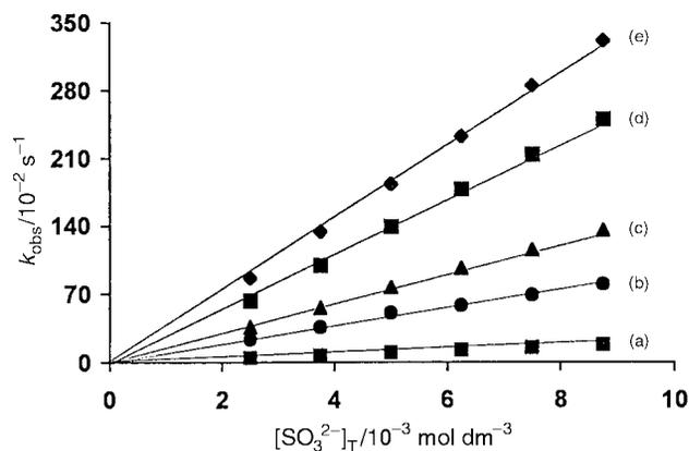
**Fig. 2** Plots of the measured first-order rate constant,  $k_{\text{obs}}$ , against [added  $\text{SO}_3^{2-}$ ] for five *S*-nitrosothiols (a) *S*-nitroso-*N*-acetylcysteine, (b) *S*-nitrosogluthathione, (c) *S*-nitrosotiopronin, (d) *S*-nitroso-2-aminoethanethiol and (e) *S*-nitrosopenicillamine.
