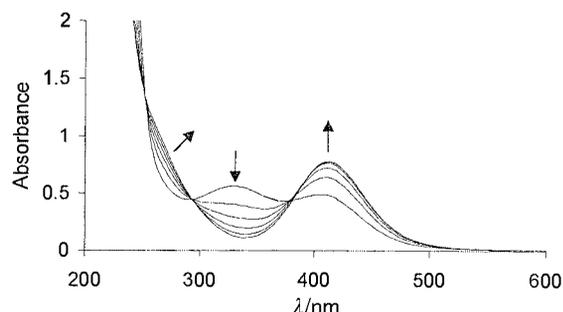
**Fig. 5** Repeat scans (every 25 s) for the reaction of GSNO (1 × 10<sup>-3</sup> mol dm<sup>-3</sup>) with sodium sulfide (1 × 10<sup>-3</sup> mol dm<sup>-3</sup>) in water (pH ~9.8) containing EDTA (1 × 10<sup>-4</sup> mol dm<sup>-3</sup>).
