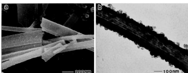
**Fig. 3** (a) SEM and (b) TEM pictures of the silica obtained from ethanol organogel **2** after calcination.
