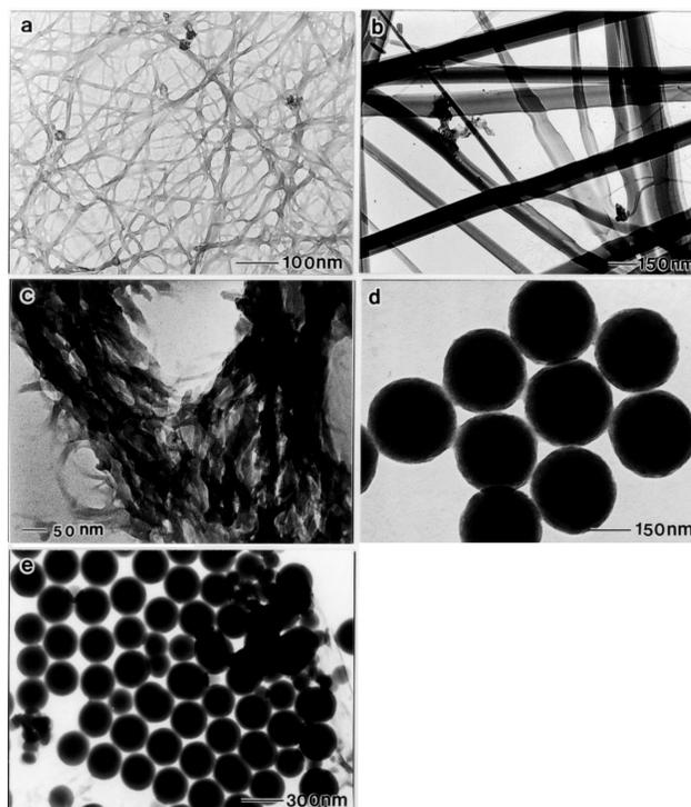
**Fig. 1** TEM pictures of xerogels: (a) 1 + EtOH, (b and c) 2 + EtOH, (d) 3 + water and (e) 4 + water. In (c), the organogel was stained with OsO<sub>4</sub> before the organogel fiber developed.
