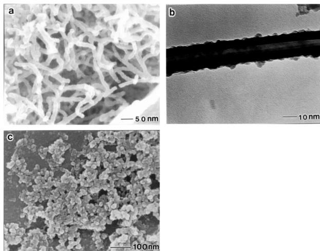
**Fig. 2** (a) SEM and (b) TEM pictures of the silica obtained from ethanol organogel **1** and (c) SEM picture of the silica obtained from ethanol gel **5**.
