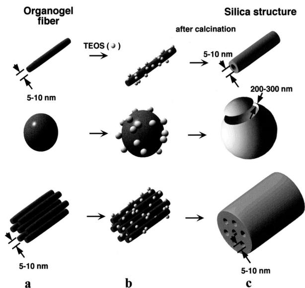
**Fig. 5** Schematic representation of the creation of various silica structures from the organogel state of **1** (upper), **2** (middle) and **3** (lower) by sol-gel polymerization: (a) gelators; (b) sol-gel polymerization of TEOS and adsorption onto the gelators and (c) single hollow fiber structure (upper), spherical structure (middle) and lotus-like structure (lower) of the silica materials formed after calcination (SEM and TEM pictures in Figs. 2, 3 and 4 were taken at this stage).
