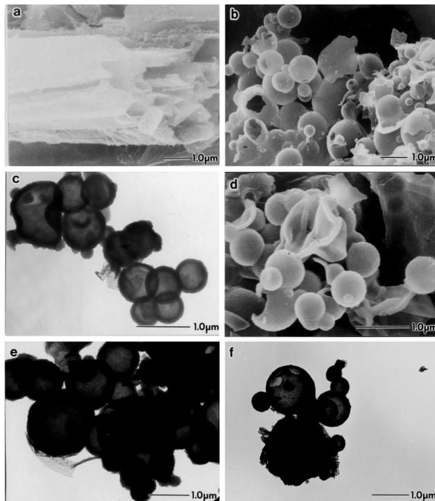
**Fig. 4** SEM pictures of the silica obtained from (a) ethanol gel **3** and (b) water gel **3**, (c) TEM picture of the silica obtained from water gel **3** after calcination, (d) SEM picture of the silica obtained from water gel **4** after calcination and TEM pictures of the silica obtained from water gel **4** (e) before and (f) after calcination.
