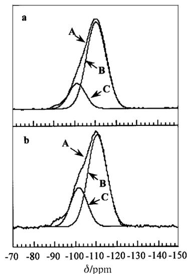
**Fig. 7**  $^{29}\text{Si}$  MAS NMR spectra of the silica obtained from (a) ethanol gel **1** and (b) aqueous gel **3**. (A) experimental curve, (B) the deconvoluted  $\text{Q}^4$  and (C)  $\text{Q}^3$ .
