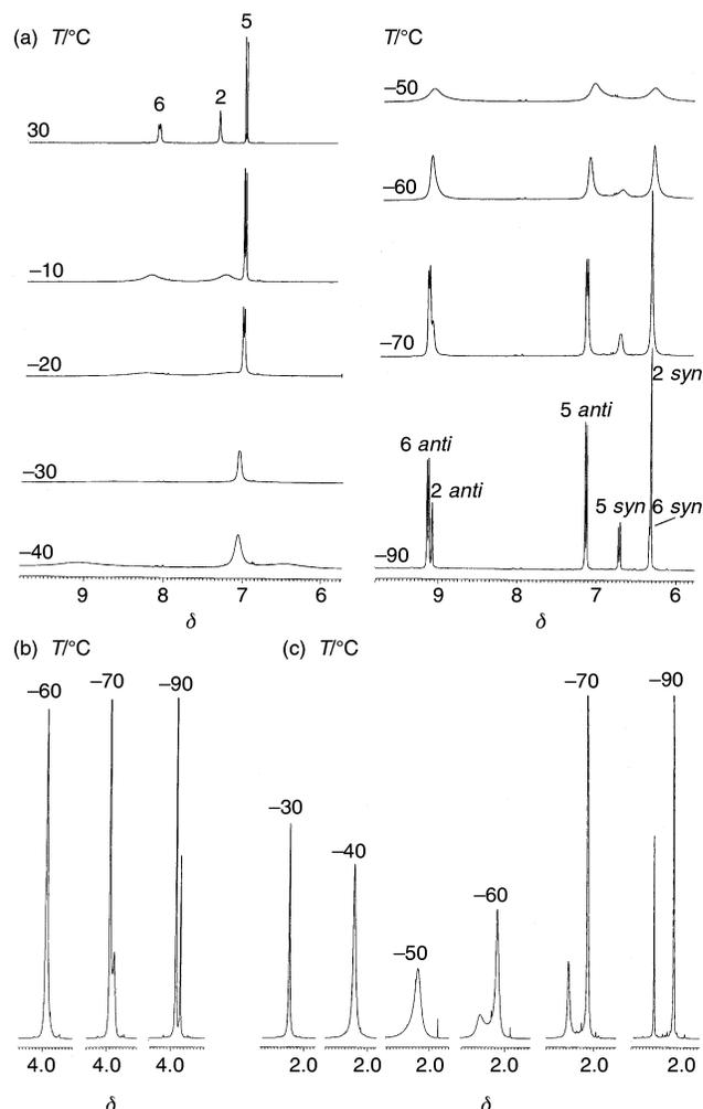
**Fig. 3** Variable temperature  $^1\text{H}$  NMR spectra of 3-methyl-4-methoxynitrosobenzene (**5**) in  $\text{CD}_2\text{Cl}_2$  showing the effects of ‘freezing out’ the  $\text{N}=\text{O}$  rotation on (a) the aromatic signals, (b) the methoxy signals and (c) the methyl signals.
