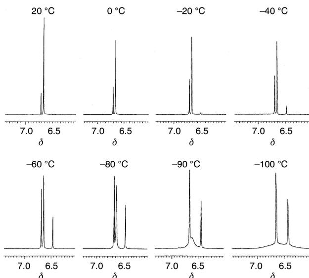
**Fig. 2** Variable temperature  $^1\text{H}$  NMR spectra of the aromatic signals of 2,6-dimethyl-4-methoxynitrosobenzene (**2**) in  $\text{CD}_2\text{Cl}_2$  showing the formation of *Z*- and *E*-dimers on cooling. At temperatures below  $-80\text{ }^\circ\text{C}$  the monomer signal broadens as a result of the slowing up of the  $\text{N}=\text{O}$  rotation.
