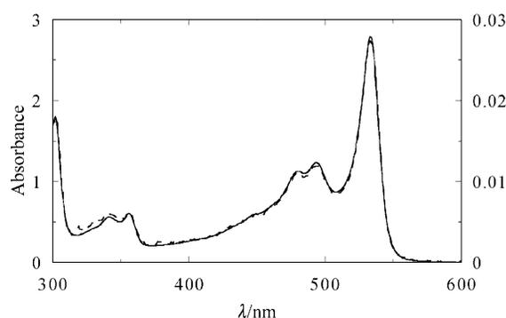
**Fig. 5** Absorption spectra of polyDCHD-HS in benzene at 20 °C. Polymer concentration:  $5.5 \times 10^{-7}$  M (full line, left scale),  $5 \times 10^{-7}$  M (dashed line, right scale).
