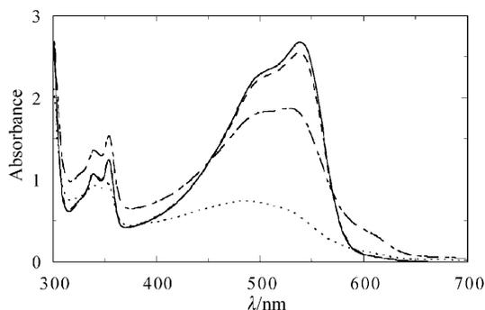
**Fig. 2** Room-temperature absorption spectrum of polyDCHD-HS in tetrahydrofuran; fresh solution (full line); after 5 days (dashed line), 15 days (dashed-dotted line); after filtration (dotted line).
