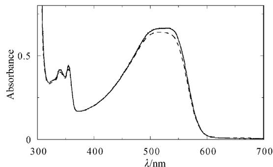
**Fig. 10** Absorption spectra of polyDCHD-HS in chloroform at different temperatures:  $T = 25$  (full line), 55 °C (dashed line); spectrum after returning to 25 °C (dotted line).
