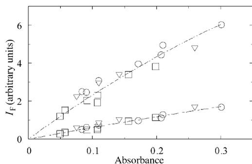
**Fig. 14** Fluorescence intensities of polyDCHD-HS in benzene at 25 °C measured at 542 nm (upper curve) and at 587 nm (lower curve) vs. absorbance at the excitation wavelengths: 480 nm (circles), 450 nm (squares), 334 nm (triangles).
