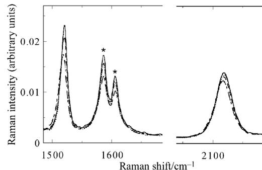
**Fig. 8** FT-Raman spectra of a benzene solution of polyDCHD-HS at different temperatures in the regions of the C≡C and C=C stretching modes:  $T = 30$  (full line), 40 (dashed line), 60 °C (dashed-dotted line); spectrum after returning to 30 °C (dotted line). Benzene lines (\*).
