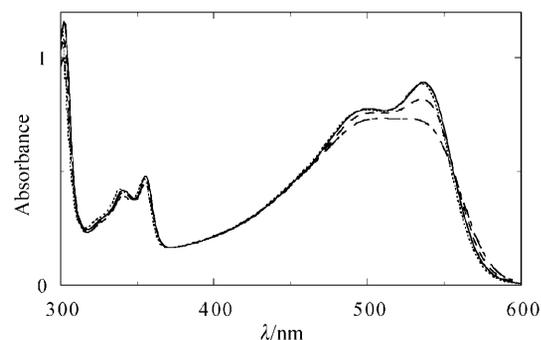
**Fig. 9** Temperature dependence of the absorption spectrum of polyDCHD-HS in toluene:  $T = 25$  (full line), 40 (dashed line), 77 °C (dashed-dotted line); spectrum after returning to 25 °C (dotted line).
