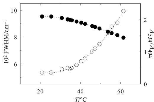
**Fig. 7** Temperature dependence of the width, FWHM (empty circles) of the excitonic peak and of the ratio of its absorbance relative to its nearest vibronic band,  $A_{534}/A_{494}$  (filled circles).
