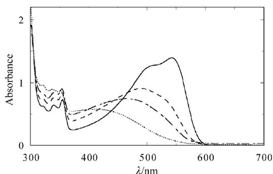
**Fig. 3** Room-temperature absorption spectrum of polyDCHD-HS in carbon tetrachloride; fresh solution (full line); after 6 days (dashed line), 10 days (dashed-dotted line), 2 months (dotted line).
