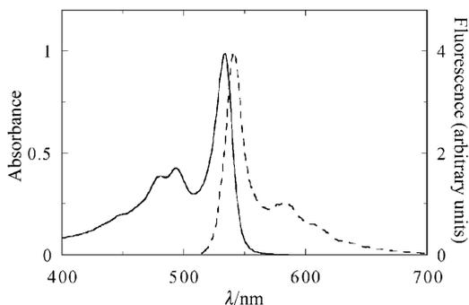
**Fig. 11** Comparison of the fluorescence emission spectrum with the electronic absorption in the visible spectral region of polyDCHD-HS in benzene at 20 °C.
