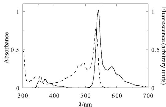
**Fig. 15** Absorption (dashed line) and fluorescence (full line) spectra of polyDCHD-HS in benzene at 25 °C for  $\lambda_{\text{ex}} = 334$  nm. The emission spectrum in the range 340–450 nm is due to the carbazolyl groups.
