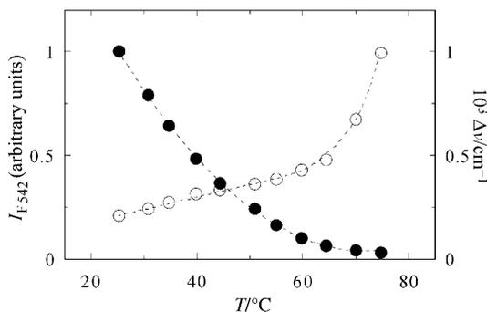
**Fig. 13** Temperature dependence of the fluorescence intensity maximum,  $I_{\text{max}}$  (filled circles) and of the Stokes shift,  $\Delta\nu$  (empty circles) of polyDCHD-HS in benzene.
