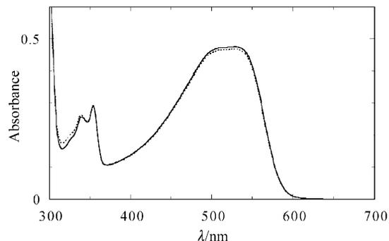
**Fig. 4** Absorption spectra of polyDCHD-HS in chloroform at 20 °C; fresh solution (full line), after filtration through a 0.2  $\mu\text{m}$  membrane (dotted line).
