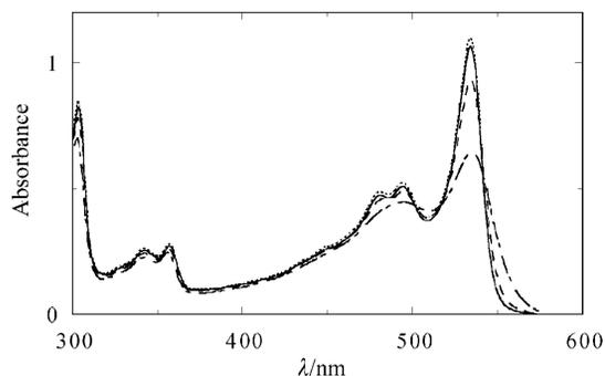
**Fig. 6** Temperature dependence of the absorption spectrum of polyDCHD-HS in benzene at  $T = 25$  (full line), 40 (dashed line), and 60 °C (dashed-dotted line); spectrum after returning to 25 °C (dotted line).
