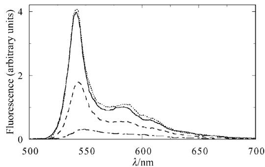
**Fig. 12** Fluorescence spectrum of polyDCHD-HS in benzene at  $T = 25$  (full line); at 40 (dashed line) and at 60 °C (dashed-dotted line); spectrum after returning to  $T = 25$  °C after heating up to 75 °C (dotted line).
