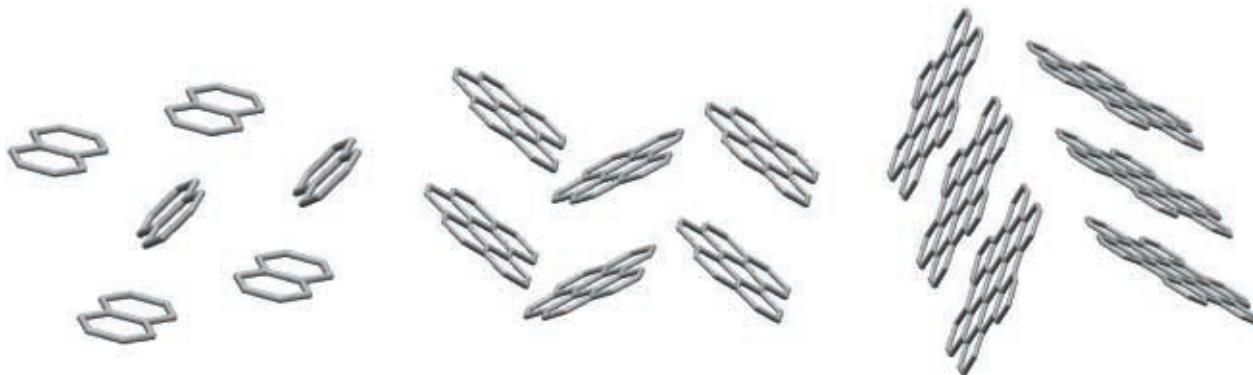
Fig. 10 Packing of naphthalene (HB, left), benzperylene (SHB, middle) and hexabenzocoronene ( \gamma -SHB, right).
