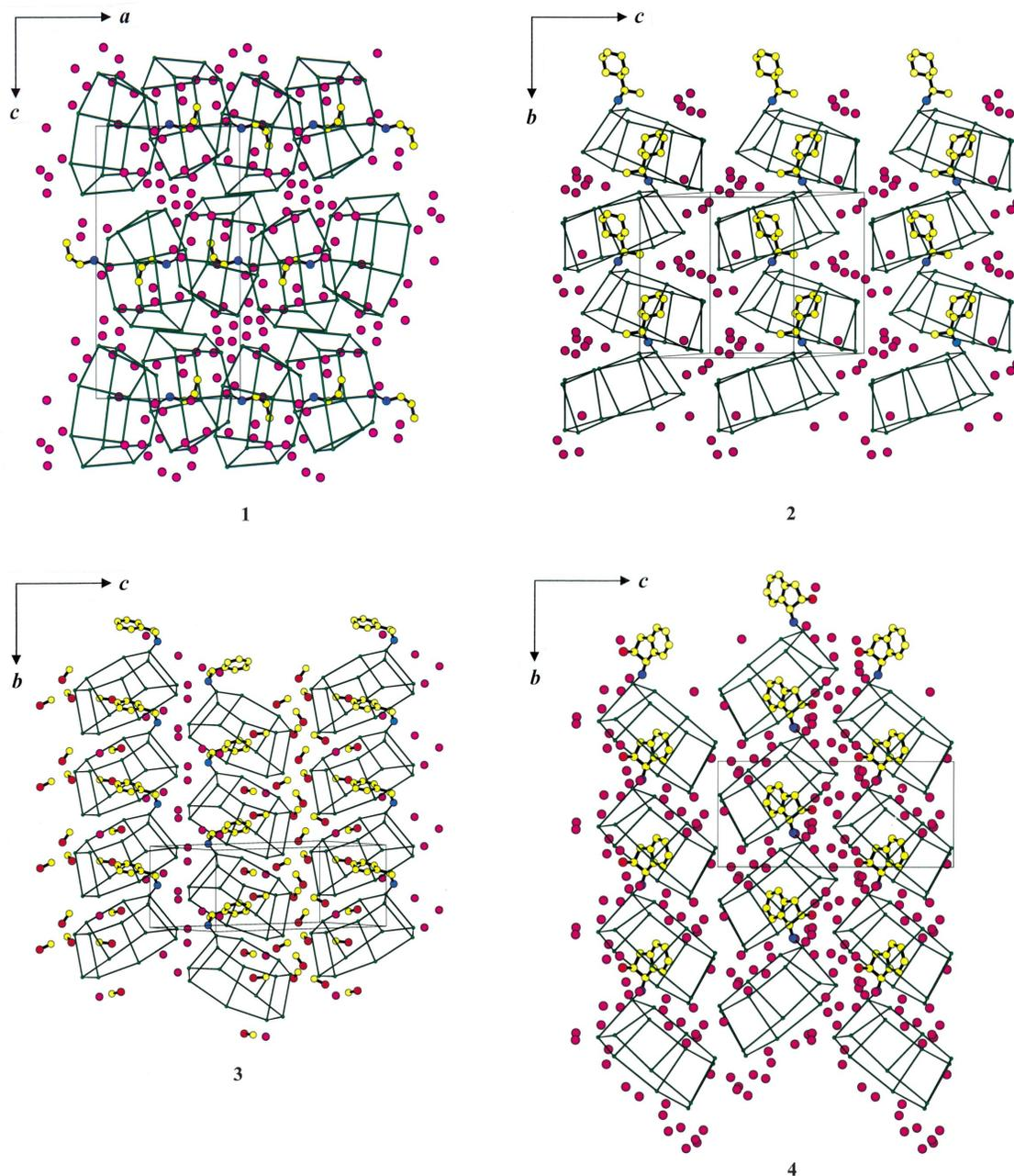
**Fig. 7** Crystal structures of the four compounds, 1–4. The  $\beta$ -cyclodextrin ring is drawn with a truncated heptagonal cone. The carbon, nitrogen, and oxygen atoms are shown in yellow, blue, and red, respectively. Water molecules are denoted by magenta circles.
