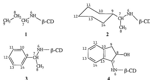
Fig. 1 Chemical structures of 6-monosubstituted  $\beta$ -cyclodextrins.
