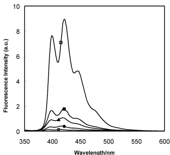
**Fig. 1** Fluorescence spectra of **5** in the absence (○) and presence of Hg<sup>2+</sup> (□), Cu<sup>2+</sup> (■), Pb<sup>2+</sup> (▲) and Zn<sup>2+</sup> (●) ions. [5] =  $1.0 \times 10^{-5}$  mol dm<sup>-3</sup>; [M<sup>2+</sup>] =  $1.0 \times 10^{-3}$  mol dm<sup>-3</sup>; in CH<sub>3</sub>OH–THF (9 : 1, v/v).
