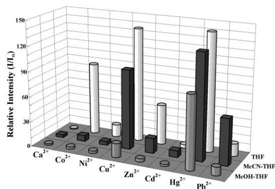
**Fig. 3** Fluorescence enhancement ratios ( $III_0$ ) of the ionophore **5** in varying solvent systems for the representative guest metal ions at 422 nm;  $\lambda_{\text{ex}} = 340$  nm. MeCN–THF and MeOH–THF denote CH<sub>3</sub>CN–THF (9 : 1, v/v) and MeOH–THF (9 : 1, v/v), respectively.
