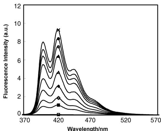
**Fig. 4** Fluorescence spectra of **5** in  $\text{CH}_3\text{OH}-\text{THF}$  (9 : 1, v/v) upon interaction with incremental  $\text{Hg}^{2+}$  ions.  $[\text{5}] = 1.0 \times 10^{-5} \text{ mol dm}^{-3}$ .  $[\text{Hg}^{2+}]/\text{5}$ : 0, ( $\square$ ); 10, ( $\blacksquare$ ); 25, ( $\diamond$ ); 50 ( $\blacklozenge$ ); 100, ( $\triangle$ ); 200, ( $\blacktriangle$ ); 300, ( $\circ$ ); 500, ( $\bullet$ ); 1000, ( $\times$ ).
