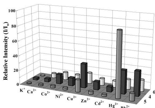
**Fig. 2** Fluorescence enhancement ratios ( $III_0$ ) for the ionophores **4–6** for the representative guest metal ions at 422 nm;  $\lambda_{\text{ex}} = 340$  nm in CH<sub>3</sub>OH–THF (9 : 1, v/v).
