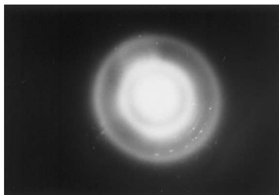
Fig. 3 Electron diffraction pattern of the dried tripeptide gel (1% w/v, camera length 0.8 m).
