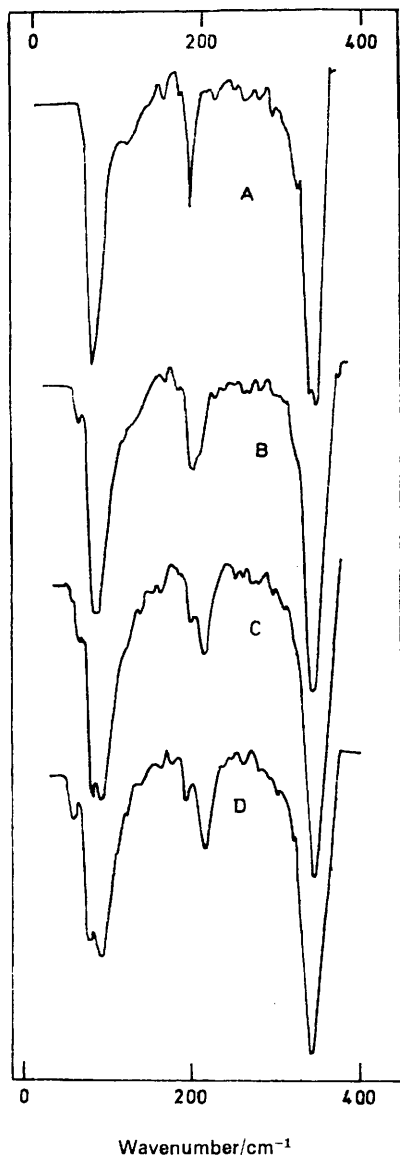
FIGURE 1 Far-i.r. spectra of \text{Cs}_2\text{PtCl}_6 at high pressures. Where doublets are shown, the lower component is the residual due to material at ambient pressure; A, Ambient pressure; B, 10 kbar; C, 15 kbar; and D, 20 kbar
