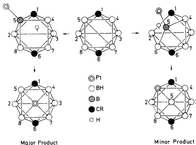
SCHEME Possible mechanisms in the reaction between 1,6- $R_2$ -1,6- $C_2B_6H_8$  and zerovalent platinum(0) species
