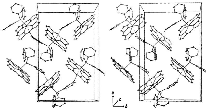
FIGURE 2 A stereopair of the crystal packing showing all atom sites. The dotted line indicates a 3.0 Å intermolecular contact of the cobalt atom with an adjacent phenyl hydrogen atom
