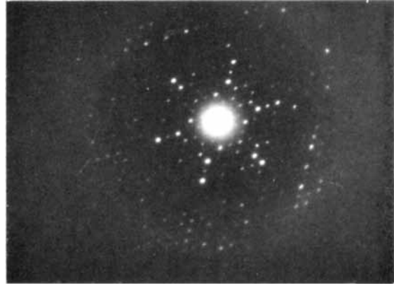
PLATE 2 Electron-diffraction pattern of zeolite ZSM2
