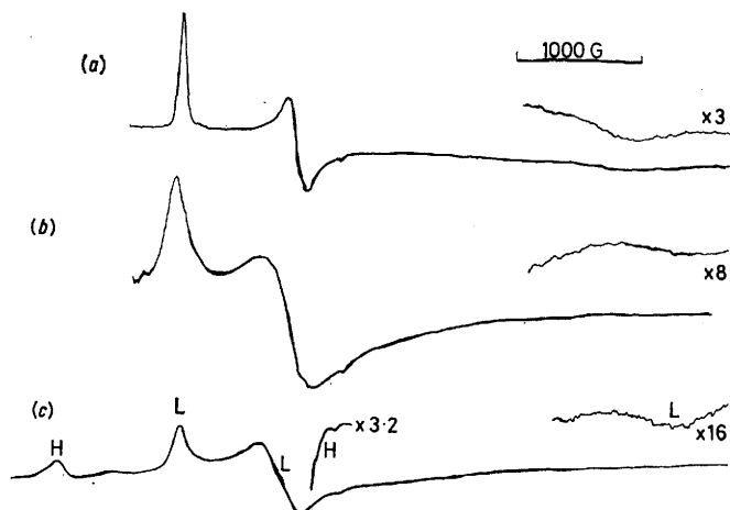
FIGURE 4 E.S.R. spectrum at 77 K of solutions containing (a) [\text{FeCl}_2\text{L}]^+ , (b) [\text{Fe}(\text{NCS})_2\text{L}]^+ , and (c) [\text{FeBr}_2\text{L}]^+
