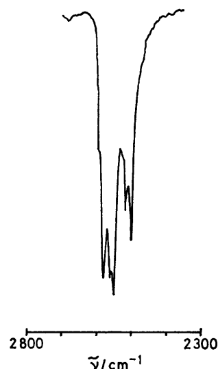
FIGURE 3 \nu(\text{B-H}) region of the solid-state i.r. spectrum of cis - [\text{Pt}(\text{B}_5\text{H}_8)\text{Cl}(\text{dppe})] (KBr disc) exhibiting strong peaks at 2580 , 2560 , 2550 , 2520 , and 2500\text{ cm}^{-1} . The spectrum of a solution in \text{CH}_2\text{Cl}_2 shows loss of fine structure to give two broader peaks with \nu_{\text{max}} at 2560 and 2520\text{ cm}^{-1}
