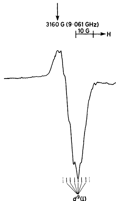
FIGURE 3 First-derivative X-band e.s.r. spectrum for \text{K}_2[\text{Ni}(\text{CN})_4] \cdot \text{H}_2\text{O} after exposure to ^{60}\text{Co} \gamma -rays at ca. 35 °C, showing perpendicular features assigned to a d^9 complex exhibiting hyperfine coupling to several ^{14}\text{N} nuclei
