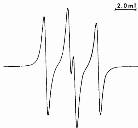
FIGURE 1 E.s.r. spectrum assigned to [\text{Fe}(\text{CO})_2(\text{L}^{\text{Me}})(\text{PEt}_3)_2]^+[\text{BF}_4]^- , (28), in \text{CH}_2\text{Cl}_2 at 20 °C
