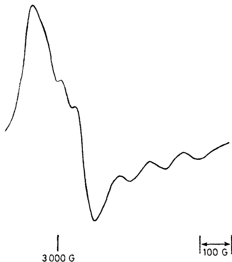
FIGURE 2 The powder e.s.r. spectrum of [\text{CuL}][\text{BPh}_4]_2
