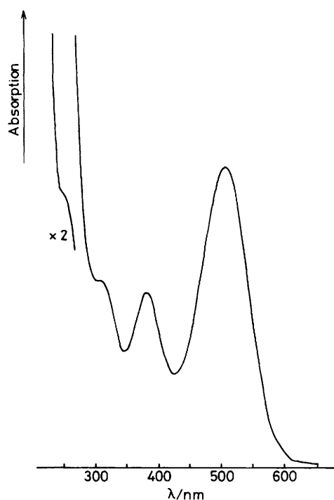
Figure 5. Electronic absorption spectrum of [\text{Fe}(\text{CO})_3(\text{bdmie})] in iso-octane
