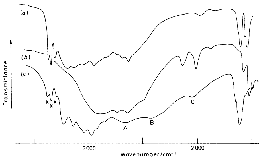
Figure 2. Hydrogen-bond i.r. spectra of (a) [N 2 H 5 ] 2 [TiF 6 ], (b) [N 2 H 6 ][TiF 6 ], and (c) [N 2 H 6 ] 2 [TiF 6 ] 2 . Bands marked with an asterisk are due to decomposition products (see text)
