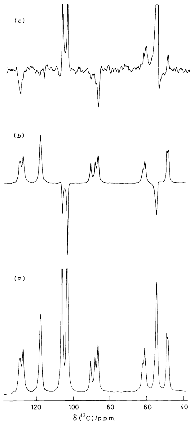
Figure. (a) A partial 100.6-MHz ^{13}\text{C} n.m.r. spectrum of [\text{Fe}(\eta^4\text{-C}_8\text{H}_8)(\text{CO})_2(\text{CNPr}^i)] in \text{CD}_2\text{Cl}_2\text{-CH}_2\text{Cl}_2 (1:1) at -118^\circ\text{C} . In addition to the cyclo-octatetraene signals there is a doublet at \delta 104.9 due to \text{CH}_2\text{Cl}_2 , a weak doublet at \delta 89.5 due to solvent impurity coincident with the signals due to carbons a' and a'' , a broad singlet at \delta 54.6 due to \text{CD}_2\text{Cl}_2 , and two signals at \delta 49.2 and 48.4 p.p.m. due to the methine carbons of the isopropyl group. (b) The partial spectrum 1 \mu\text{s} after applying a selective 180^\circ pulse at \delta 55.5 p.p.m. A side-band, 5 kHz away perturbed the \text{CH}_2\text{Cl}_2 signal. (c) A difference spectrum obtained by subtracting spectrum (b) from that obtained 10 ms after applying a selective 180^\circ pulse at \delta 55.5 p.p.m.
