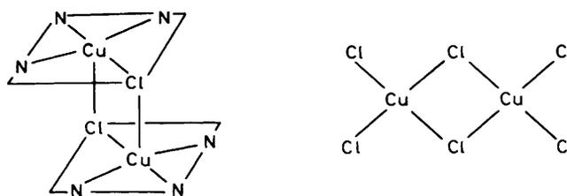
Figure 4. Proposed constitution of  $\text{Cu}_2(\text{terpy})\text{Cl}_4$ : the  $[\{\text{Cu}(\text{terpy})\text{Cl}\}_2]^{2+}$  cation and  $[\text{Cu}_2\text{Cl}_6]^{2-}$  anion
