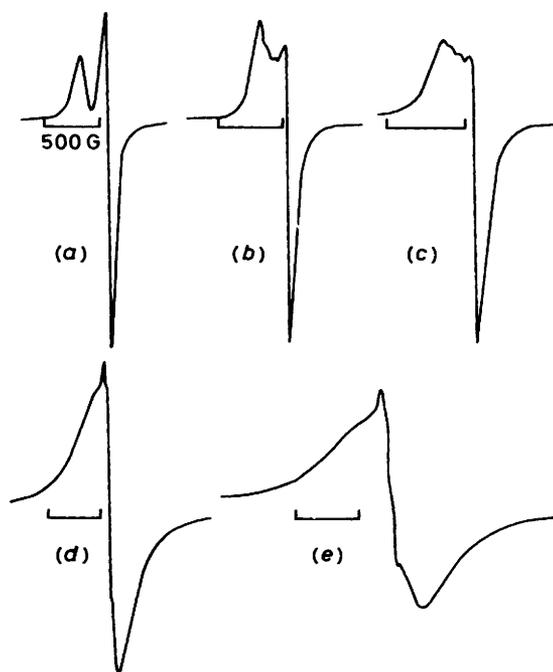
Figure 2. Temperature dependence of the e.s.r. spectrum (X-band) of  $\text{Cu}_2(\text{terpy})\text{Cl}_4$ : (a) 4 K, (b) 40 K, (c) 50 K, (d) 110 K, (e) room temperature
