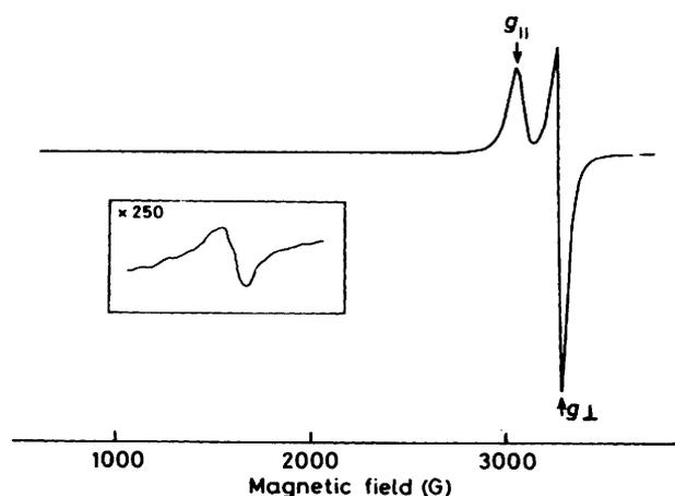
Figure 1. Polycrystalline powder e.s.r. spectrum (X-band) of  $\text{Cu}_2(\text{terpy})\text{Cl}_4$  at 4.2 K
