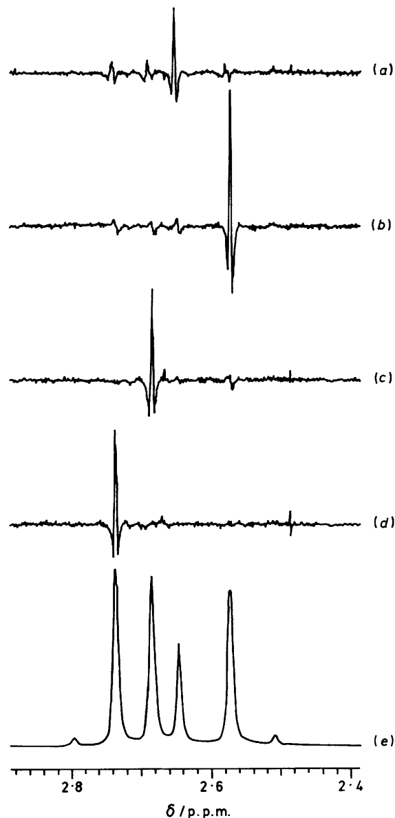
Figure 5. The ^1\text{H} decoupling difference spectra in the region 2.8–2.5 p.p.m.: irradiating at (a) 3.89 p.p.m. ( \text{H}^4 of minor species), (b) 3.49 p.p.m. ( \text{H}^4 of major species), (c) 3.62 p.p.m. ( \text{H}^{14} of major species), and (d) 4.25 p.p.m. ( \text{H}^8 of major species), (e) normal spectrum for reference
